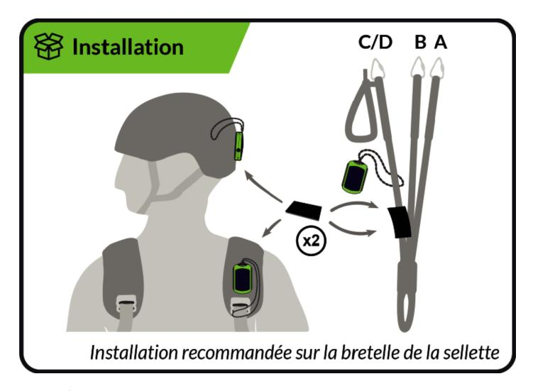
**Installation:** 2 Velcro loops are supplied with the BipBip PRO V2 to attach it to your equipment.
