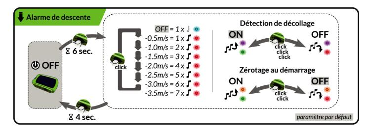
**Setting the descent alarm:** You can change the descent alarm setting at any time, even just before take-off, by following the diagram above.
