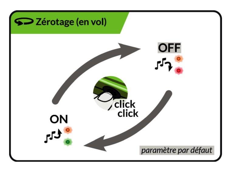
**Zerotage:** brief modulations indicating an area of very weak lift, not strong enough to roll but potentially close to a thermal (vario from -30cm/s to the selected climb rate, default +15 cm/s).
