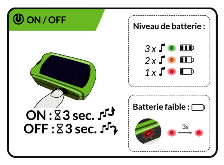
**ON:** To switch on your BipBip PRO V2, press and hold the button for 3 seconds. You'll hear the start-up melody, followed by the battery level.
